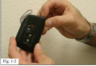
(c) Use a finger to position the elastic band over the top edge of the remote (Fig. 1-2).
